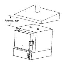
A Vent Hood is recommended for burnout furnaces.
